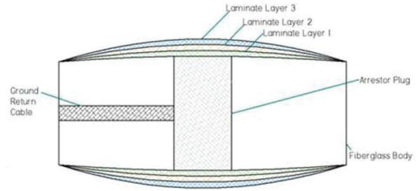
While the average lightning strike discharges 30-50 kA, NASA has recorded strikes above 100 kA and there are other reports of lightning strikes exceeding 200 kA. Testing was performed at these high amplitude conditions to prove the validity of the system.
